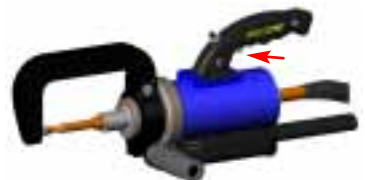
Push this button to close electrodes and weld.
