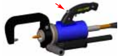
Push this button to open electrodes wide.
